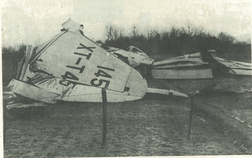
No. 10 and 11 The fuselage. The pictures show how flat the plane crushed by coming down flat.
